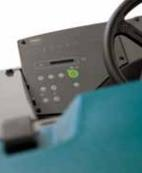
Optional 1-Step<sup>™</sup> start button simplifies operator training with controls that enable sweeping systems to be activated with a single green button
