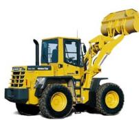
provides better visibility, increased comfort, see-at-a-glance console, two-door walk-through and finger-touch shifting. See page 4. New special rubber-mounted cab for productivity. Special rubbermounted cab reduces vibration and noise that can fatigue the operator and reduce his efficiency. See page 4.
