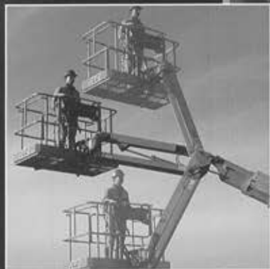
Articulating Jib Provides Reach Versatility
