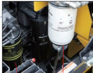
Fuel filter Fuel pre-filter (with water separator)
